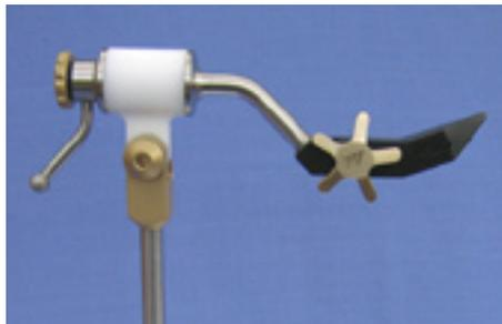
The LAW vice is a full 360° horizontally rotating vice. The jaws will securely hold any hook from 7/0 down to 28 and smaller, with one adjustment only. The vice is provided with a pedestal base or a C-clamp, and comes with an articulated bobbin holder. Several optional accessories are available. These are listed in the Options section of this guide.
