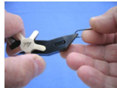
Rotate the Star Wheel to fasten the hook. While the design is based on intuitive thumb-only operation, some tiers prefer to operate the Star Wheel with thumb and fingers. Try the various methods and select the one which works best for you.
